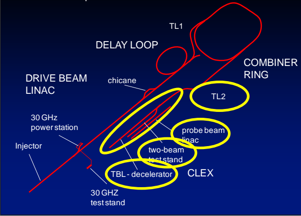
CTF3 – Main components
