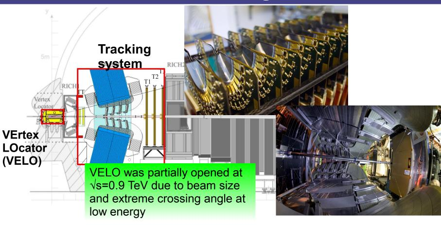
$δp/p \sim 0.5\%$  - reconstruction efficiency ~95% Resolution for primary(secondary) vertices is  $σ_z \sim 50(150) \mu m$
