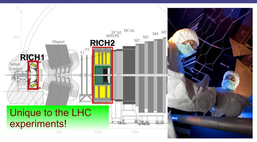
2 Ring Imaging CHerenkov (RICH) detectors provide charged particle identification in a momentum range of 2 - 100 GeV
