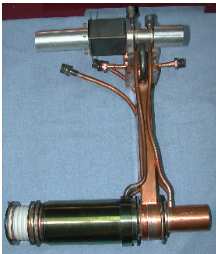
X-band 2.5MeV SW Tube Powered by a 1MW 9300MHz magnetron
