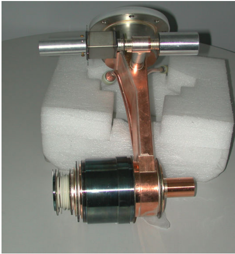
S-band 2.5MeV SW Tube Powered by a MG5125 magnetron
