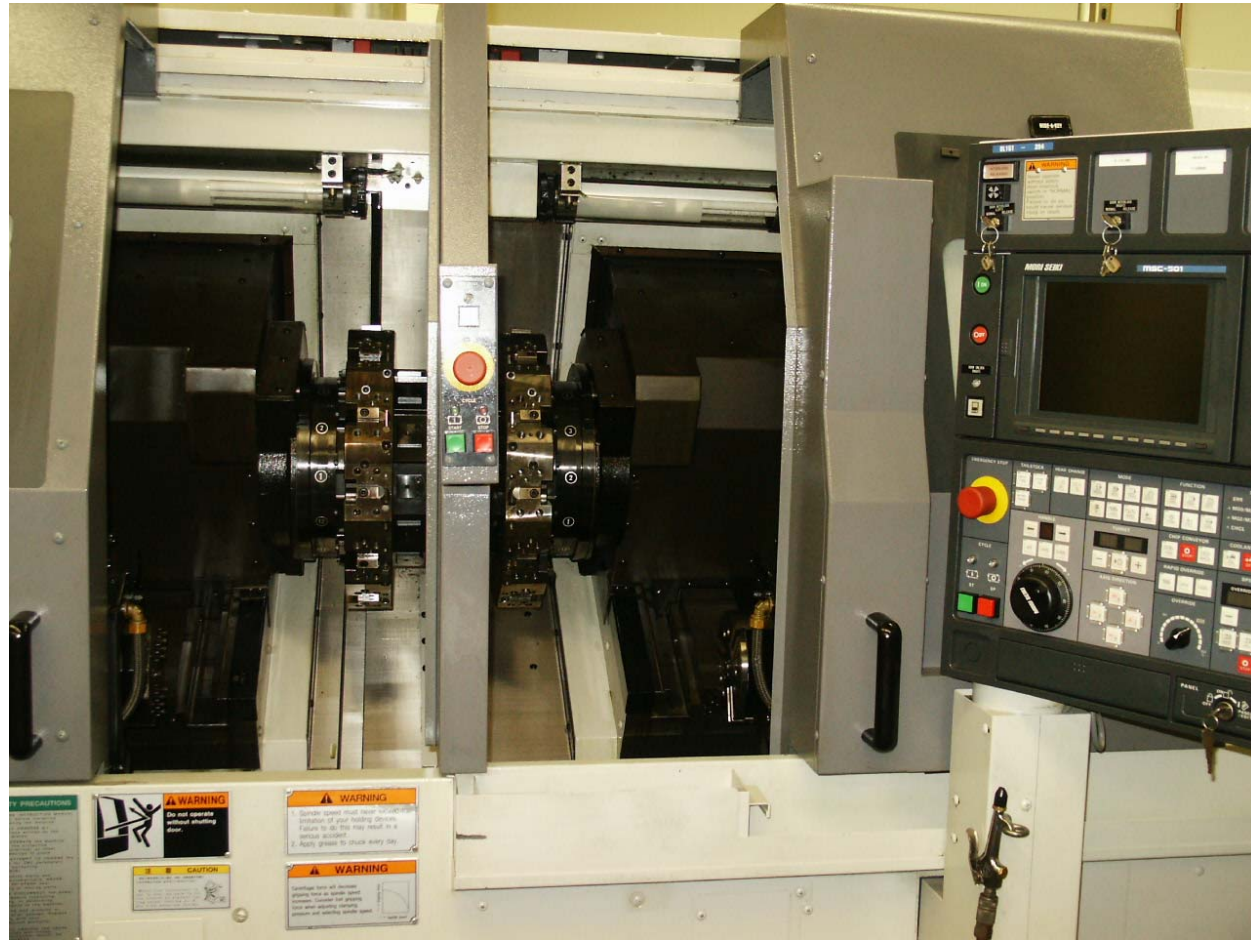
Lathe with Twin Spindles and Twin Turrets Profile tolerance 5 \mu\text{m} and Surface finishing 300 - 400 nm
