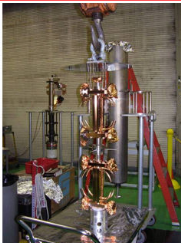
Vacuum Baking of T18_vg2.4_DISC
