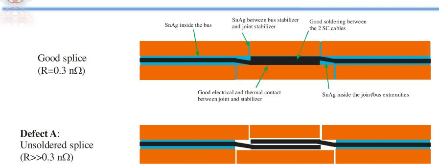
Defect A is very likely to be found using the monitoring feature of the nQDS system, which should reveal all bad splices with a resistance larger than a few n $\Omega$ .
