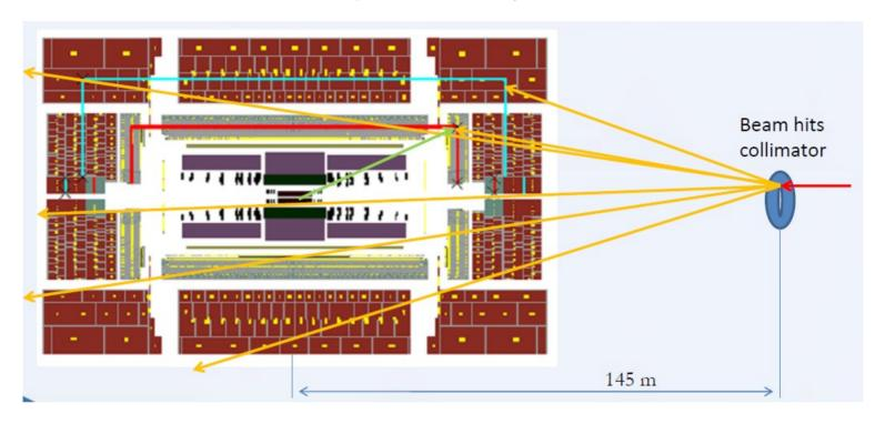
Splash events occur when beam is hitting collimator:
