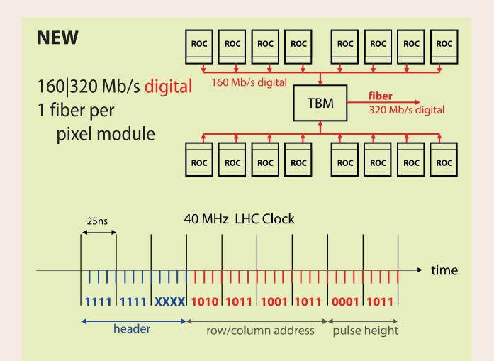
Each ROC will deliver digital data at 160 Mb/s and the TBM will produce a multiplexed signal train at 320 Mb/s. One half-stream will be inverted in order to generate a NRZ signal which is suitable for optical transmission.
