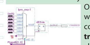
Our approach is to sample the incoming serial data with several different clock phases (this essentially corresponds to oversampling), histogram the transitions between adjacent samples and pick the clock phase with maximum distance to transitions.
