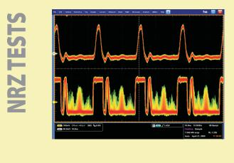
Heavily unbalanced **code** (here: 1000 0000 = 12.5% duty cycle) is correctly identified by the optical head (top), but not by the Zarlink receiver (bottom).
