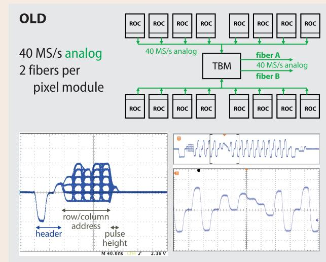
Left: eye diagram of **ROC output** data. After the header (negative peak), the pixel address is coded using analog levels, followed by the analog pulse height.
