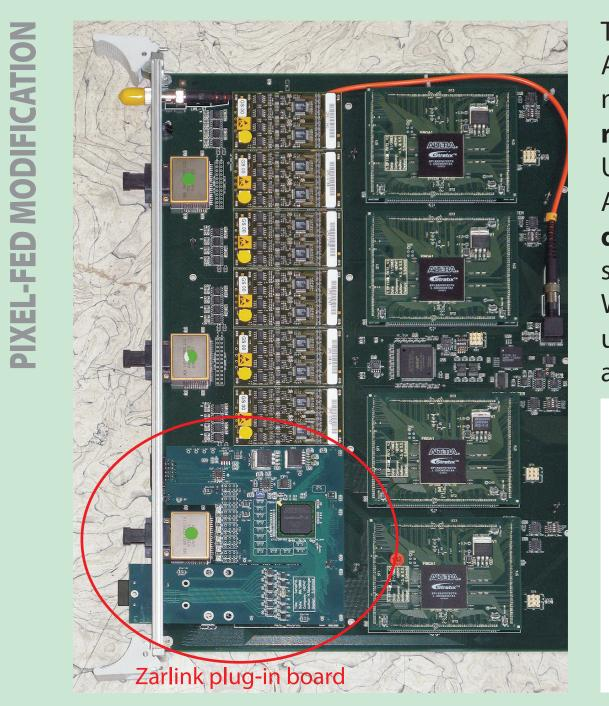
The present Pixel-FED contains three 12-way analog receivers and  $3 \times 3=9$ ADC daughter boards. Obviously, neither analog receiver nor ADCs are needed anymore when going digital, while it would be economical to retain all the other parts of the Pixel-FED.
