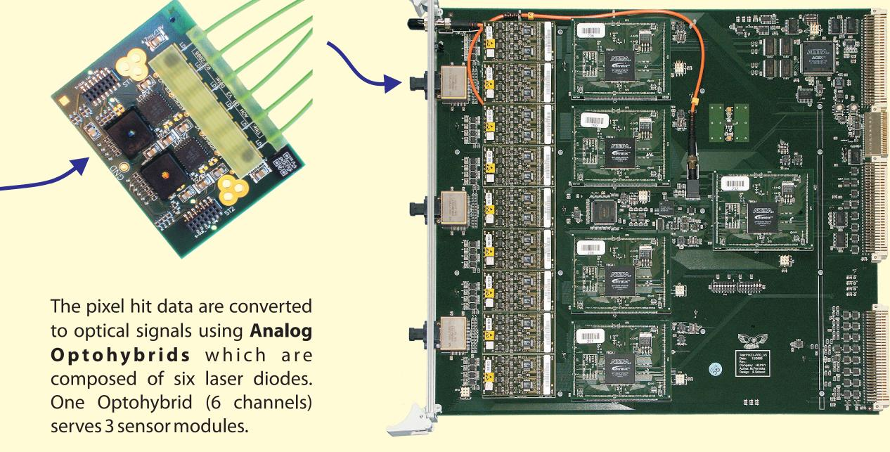
32 of these 9U VME Pixel-FED modules serve the barrel part, 8 more are used in the forward section. A 6U S-Link board is attached to the rear of each Pixel-
