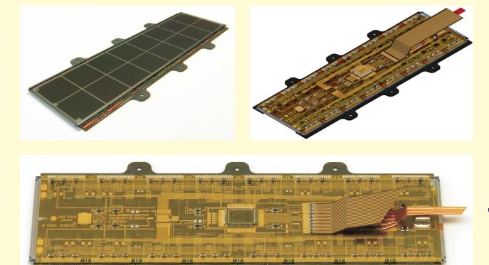
A **barrel sensor** (shown here) is read out by 16 Readout Chips (ROCs), a forward sensor needs 24 ROCs. The pixel data are collected by the central Token Bit Manager (TBM) and transmitted to the Analog Optohybrids over controlled impedance differential lines.
