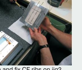
Align and fix CF ribs on jig2
