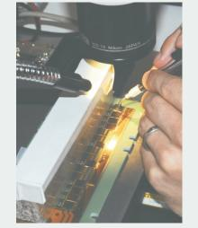
Attaching APV25 chips (gluing, wire bonding)
