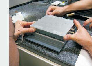
Put ribs together with jig2 onto jig1 and flip the module
