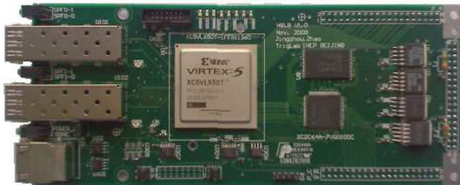
DSP Belle2link Receiver Prototype
