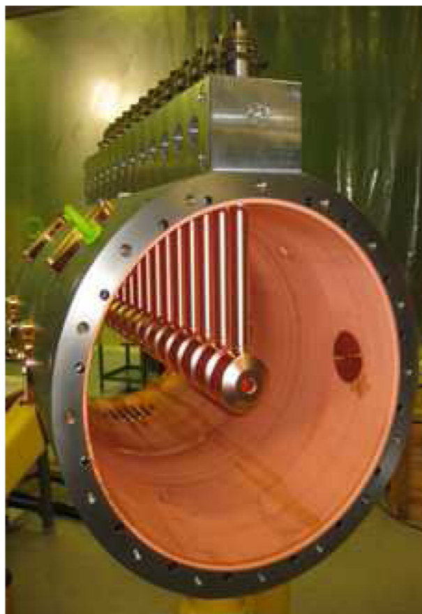
Figure 4: DTL prototype in the assembly stage.
