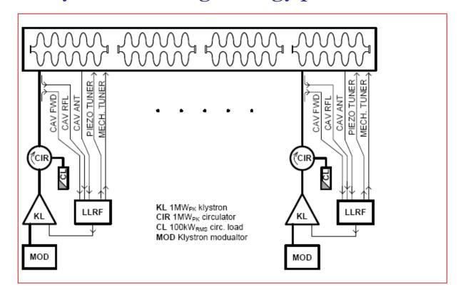
I klystron per cavity: individual control possible without RF vector modulator Disadvantage: Many klystrons required
