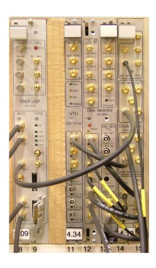
modified LHC hardware: four channels analog down conversion to IF
