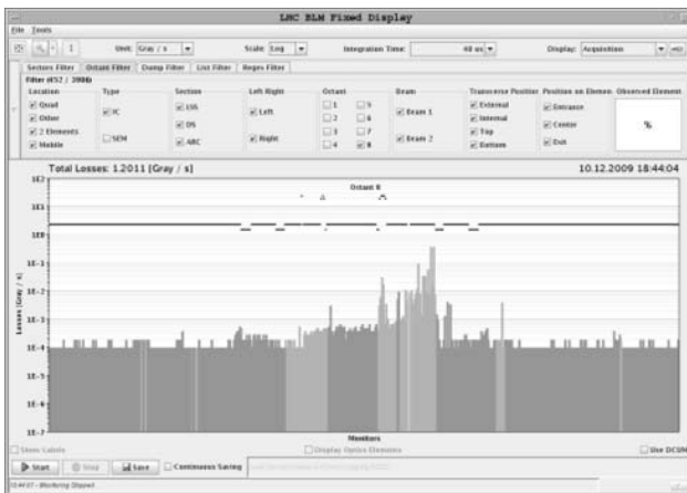
Figure 3: Losses in the B2 injection area for a pilot bunch with 5 \cdot 10^9 protons and horizontal transfer line collimators at 6 \sigma (hor) and 4.5 \sigma (vert).
