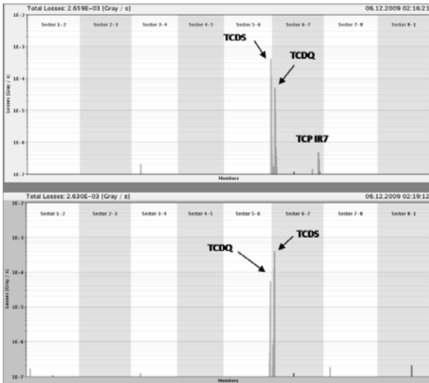
Figure 7: Losses on the dump protection devices TCDQ and TCSG for B1 (top) and B2 (bottom).
