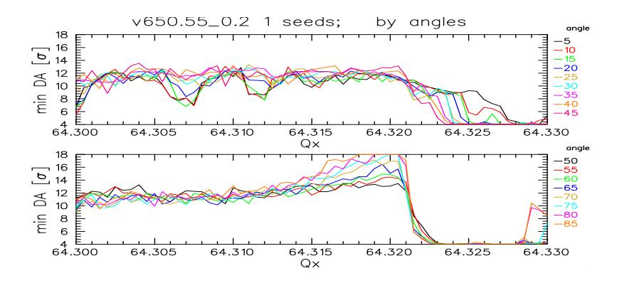
Dynamic aperture: tune scan with beam-beam for the LHC ...
