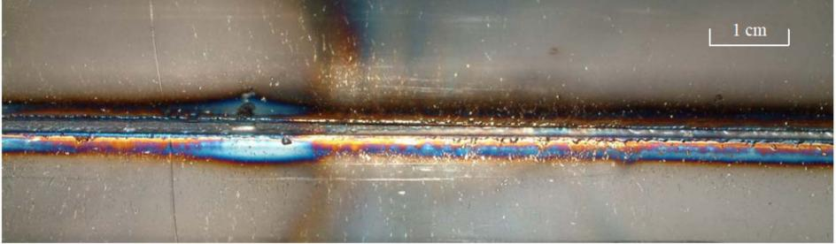
Figure 4. Damage observed on the inside of the vacuum chamber, on the beam impact side. A groove approximately 110 cm long due to removed material was clearly visible, starting at about 30 cm from the entrance.
