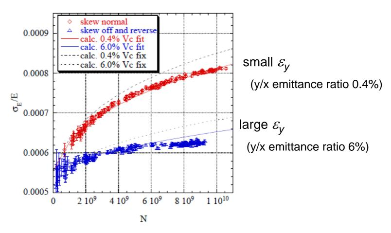
Calculation with fitted *Vc* (which was fitted to reproduce measured bunch length) agree with measured momentum spread data much better than fixed VC.
