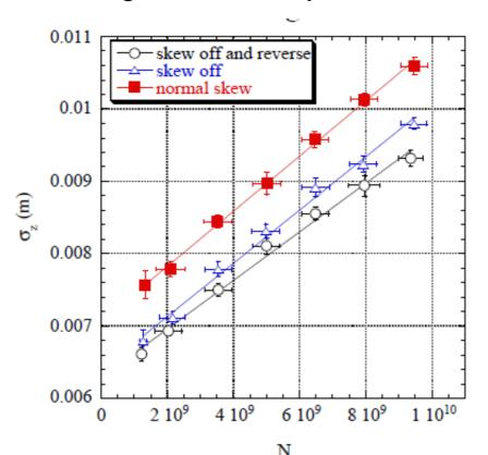
Strong intensity dependence even for large vertical emittance, where IBS should be very weak.
