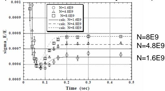
Longitudinal damping time ~ 1/2 vertical damping time.
