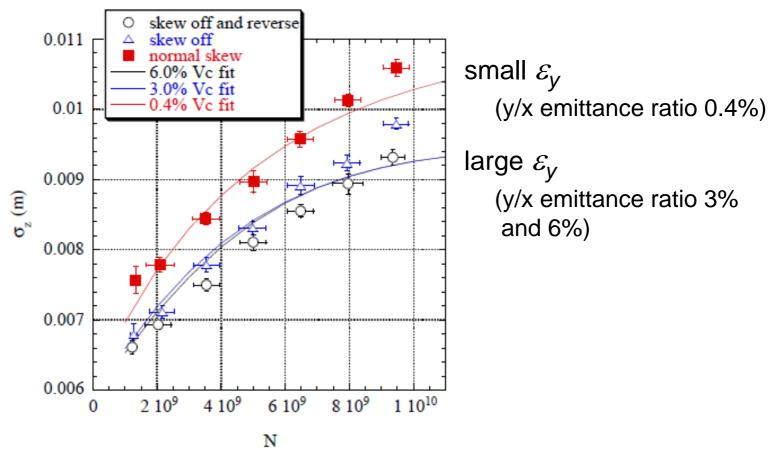
Difference between calculation and measurement may come from noninductive components of impedance.
