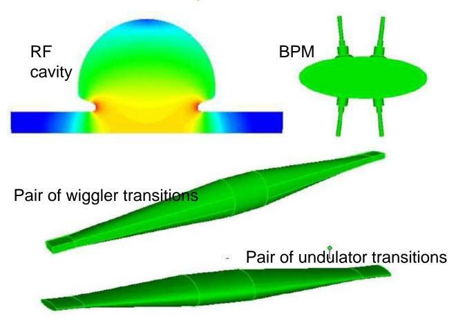
Selected impedance objects included in our straw man PEP-X design. Note: the fundamental mode fields are shown in the RF cavity.
