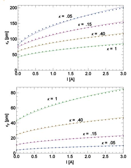
Steady-state emittances as function of current in PEP-X for various couplings. Dots give the solution to the fitted 1d equation.
