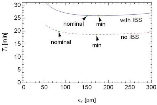
Touschek lifetime as function of  $\varepsilon_x$ , with  $\varepsilon_y$ ,  $\sigma_p$  fixed. This is not a self-consistent calculation. (The lattice is for a slightly earlier version of PEP-X.)
