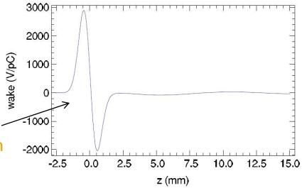
Haissinski solution, giving the steady-state bunch shape. Bunch length is 25% above nominal length.
