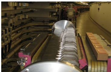
FIGURE: New chamber in modified quadrupole QN9.
