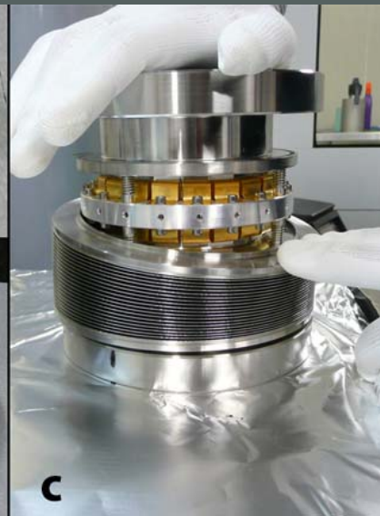
gold coated strip (a), supporting Al ring (b), bellows assembly (c).
