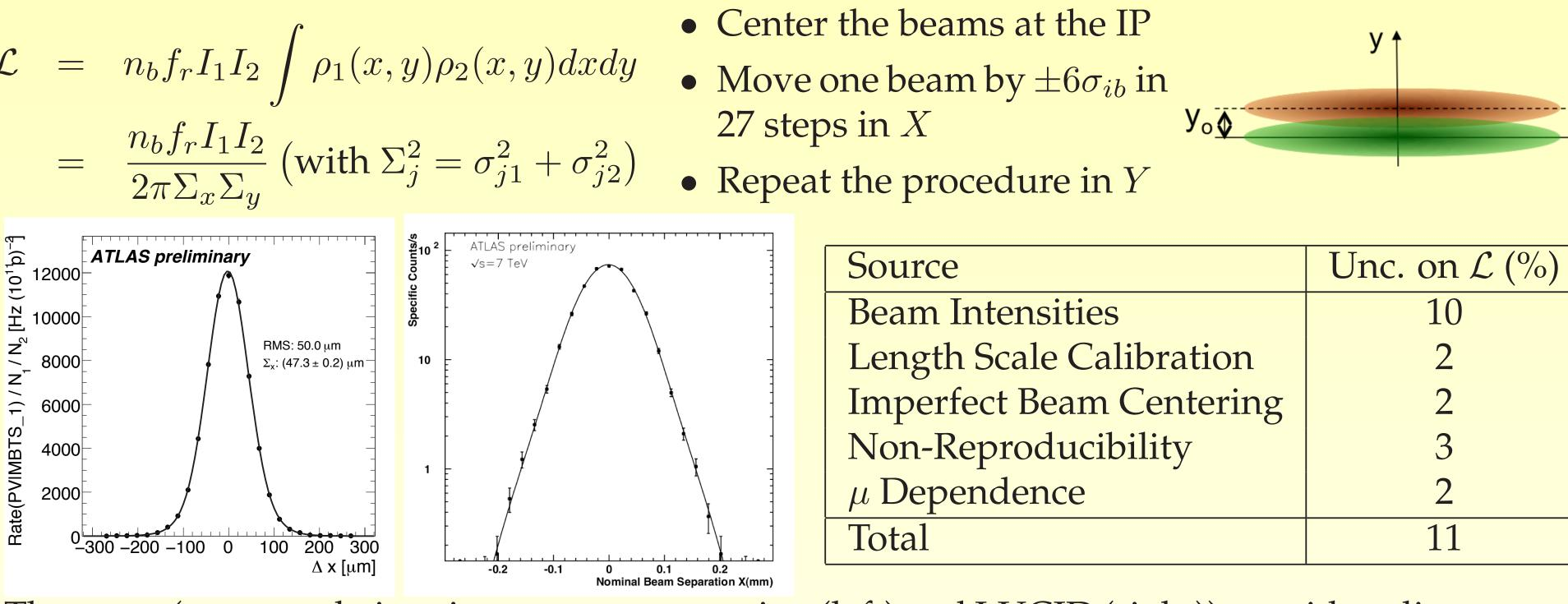
The scans (measured via primary vertex counting (left) and LUCID (right)) provide a direct measure of the absolute luminosity of the LHC, and a factor  $\times 2$  precision over Monte Carlo calibrations.
