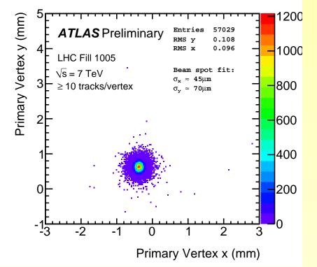
Offline primary-vertex distributions in the *x*-*y* plane, uncorrected for resolution, at  $\sqrt{s} = 7 \text{ TeV}$
