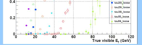
The above plot shows the trigger efficiency for taus which are also reconstructed offline for various trigger items (produced from  $Z \rightarrow \tau \tau$ Monte Carlo Simulation).
