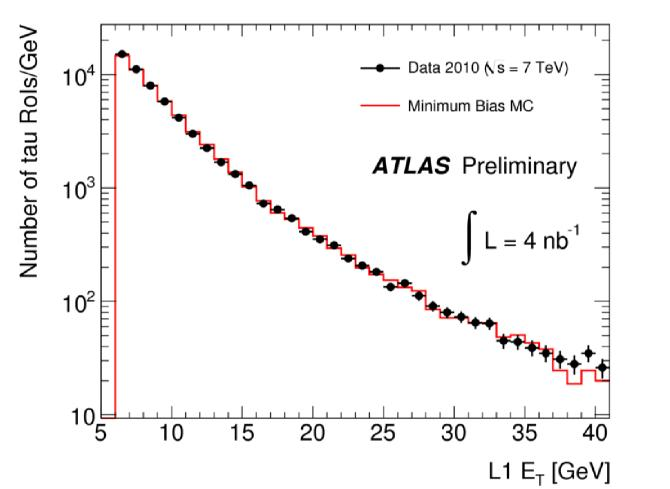
These plots show a comparison between 7 TeV data and Minimum Bias MC for important quantities at each level of the tau trigger.
