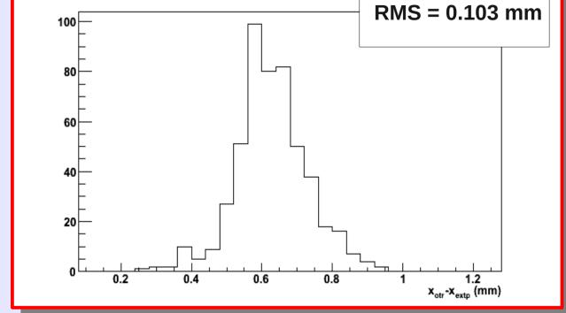
The difference between the OTR measurement and a fit to upstream monitors gives a measurement of the combined resolution: 100  $\mu$ m or bettter for the position measured by OTR.
