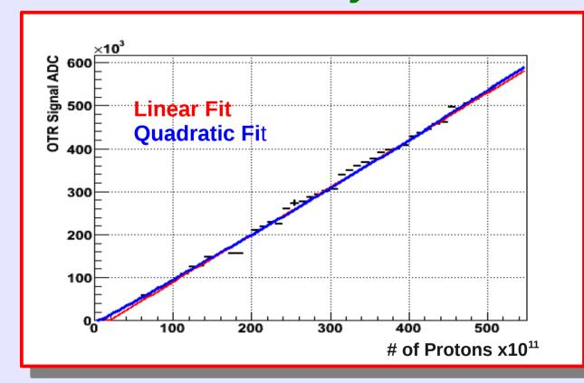
The total OTR light (integrated ADC counts) is linear with the number of protons traversing the foil, as expected.
