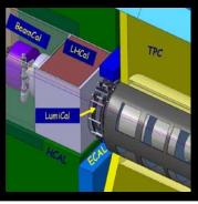
Two types of sensor materials are considered: GaAs (most of BeamCal) and CVD diamond (the innermost part, adjacent to the beam-pipes).
