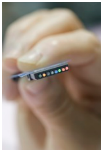
Fibers bundled into cables to interface with 64 channel multi-anode PMT's.
