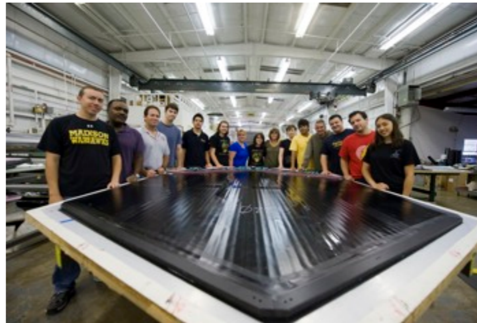
Strips are bundled into PLANES to provide transverse position location across a module.
