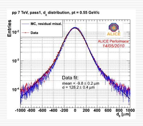
The resulting resolution is the convolution of the trackposition and the primary-vertex resolutions
