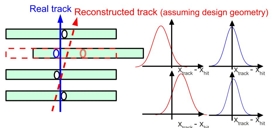
Use tracks to determine 'real' module position by minimisation of track residuals ( $\mathbf{r} = x_{track} - x_{hit}$ )
