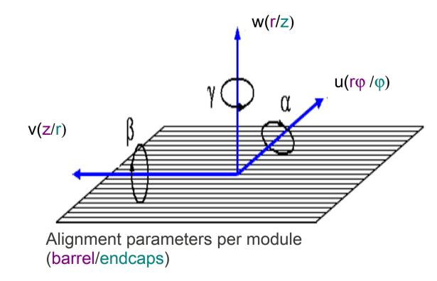
Independent from the global orientation of the module the alignment parameter u is always pointing orthogonal to the strips and is thus the most sensitive coordinate ( $r\phi$  in the barrel and  $\phi$  in the endcaps).
