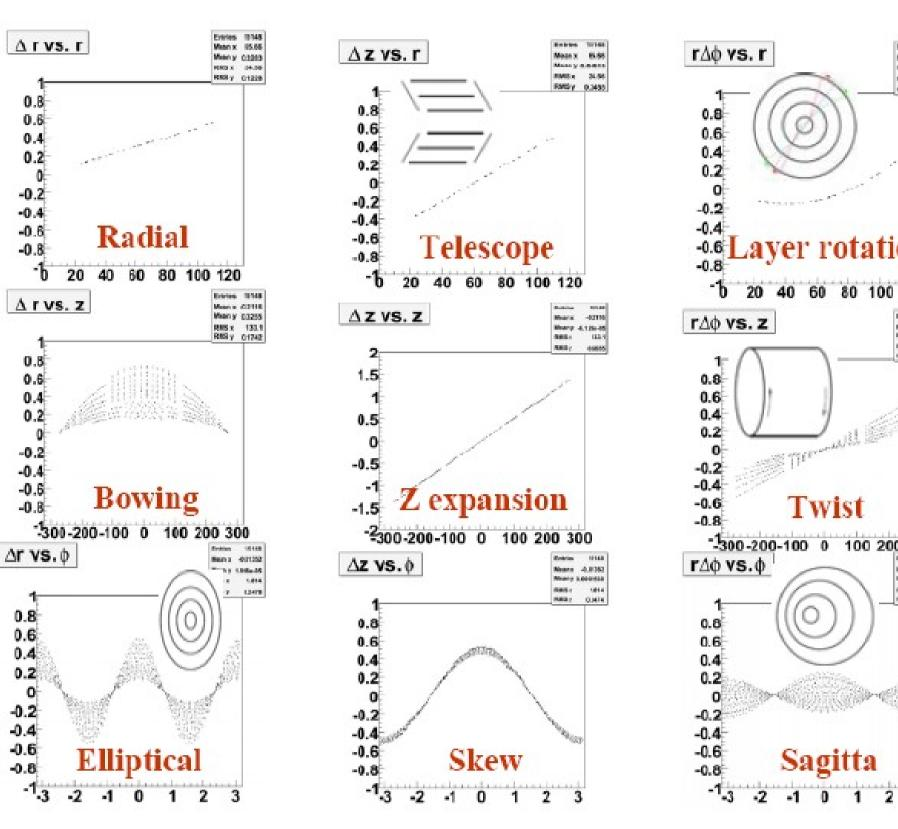
To detect and investigate the influence of possible weak modes the above correlated detector deformations were applied on top of the latest tracker geometry, then aligned back following the same strategy as before and compared to the starting geometry.
