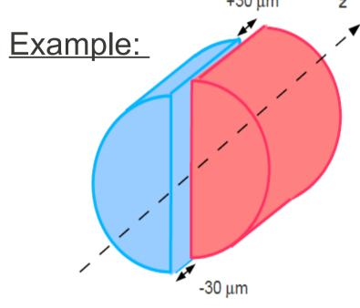
A z-shift of the two pixel half-shells by 30 micron in opposite directions would result in a shift of  $d_z$  of 30 microns for different regions in  $\phi$  as shown below.
