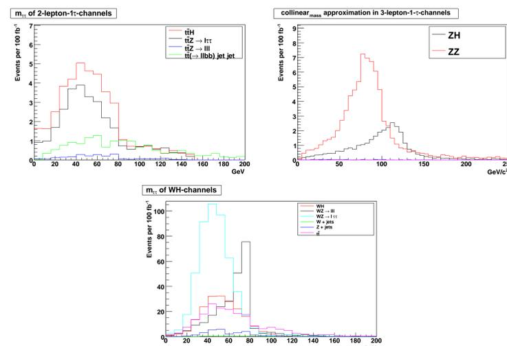
Pseudo-experiments are generated from signal and background MC distributions according to a Poisson distribution,  $P(k; \lambda) = \frac{\lambda^k \exp(-\lambda)}{k!}$ , for  $k$  observed events and  $\lambda$  expected events. The number of signal events is extracted by minimising the log-likelihood as a function of the signal yield.
