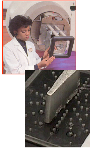
Cerrobend Blocks Electron Blocks
