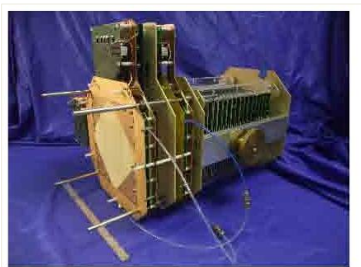
The prototype proton range telescope. The active area is 10x10cm.
