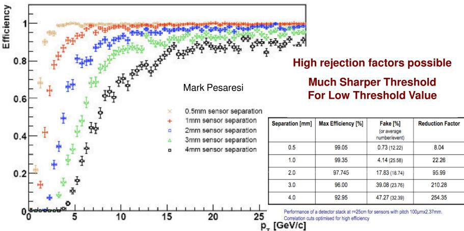
p<sub>T</sub> discriminating performance of a stacked layer at r=25cm for various sensor separations using 10,000 di-muon events with smearing
