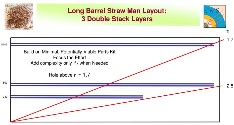
3 Double Stack L1 & Tracking Layers, with full acceptance up to  $\eta \sim 1.7$ : Each Layer provides 2 \* 2 = 4 hits 3 Layers = 12 hits Single System provides Full L1 & Tracking functionality 2700
