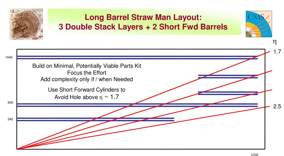
3 Double Stack L1 & Tracking Layers, with full acceptance up to  $\eta \sim 2.1$ : Each Layer provides 2 \* 2 = 4 hits 3 Layers = 12 hits Single System provides Full L1 & Tracking functionality Short FWD Cylinders close acceptance Total Silicon Surface ~ 375m<sup>2</sup> Present Tracker ~ 210m<sup>2</sup>
