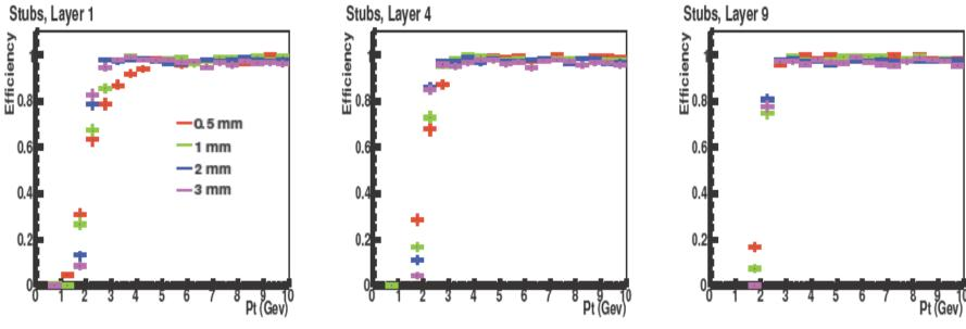
The Pt thresholds are sharper at larger radii, as expected
