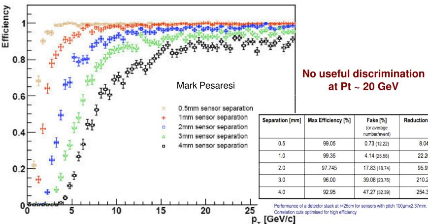
p<sub>T</sub> discriminating performance of a stacked layer at r=25cm for various sensor separations using 10,000 di-muon events with smearing
