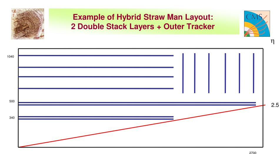
2 Double Stack L1 & Tracking Layers, with full acceptance up to  $\eta \sim 2.5$ : Each Layer provides 2 \* 2 = 4 hits 2 Layers = 8 hits Outer Tracker: Optimized for Tracking No L1 functionality Introduces 3'rd System, in two "flavors"
