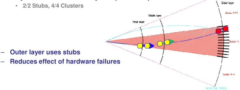
Segments must overlap due to imprecise projection
