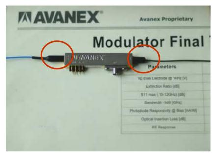
48 x 9.3 x 5.0 mm<sup>3</sup> (Excluding connections: 13 mm in + 18 mm out)
