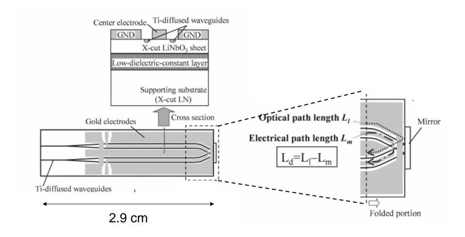
Scheme for a 40 Gb/s folded modulator proposed and fabricated by Aoki in 2007 Performance similar to standard modulators
