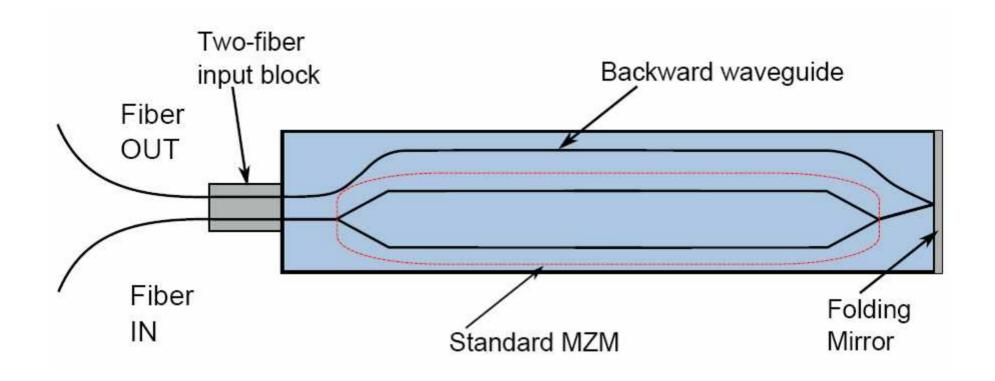
Slight modification of packaging and device in current MZM Study of packaging options for better integration on Si detector board
