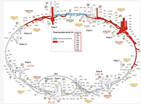
Need to implement alternative He release path to surface to get more access flexibility during tests
