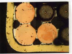
Sample Id: 6 kA hairpin connection Description: Cross-section corner 4, at crimp, lack of wetting + presence of cracks in the brazing Original magnification: 25.0 x coaxial
