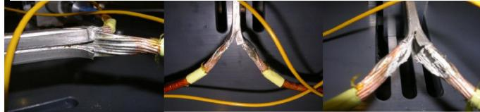
Fig.5 Electrical connection after 17190 cycles
