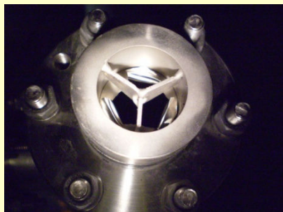
Q8R3 V2: rupture disk blown
