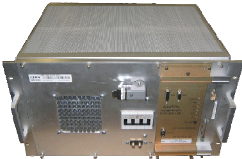
Figure 7: LHC60A-08V Power Converter
