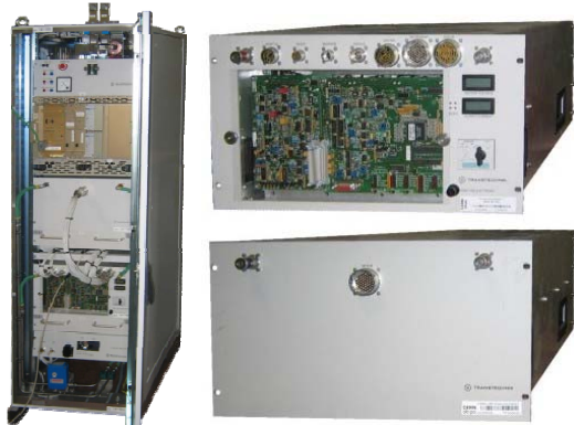
Figure 10: LHC600A-40V Power Converter
