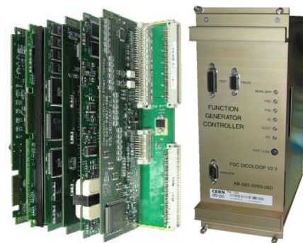
Figure 3: Function Generator Controller (FGC)
