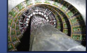
Add a new b-layer around a smaller beam pipe (in radius), stave structure, 160 MHz readout, CO<sub>2</sub> cooling
