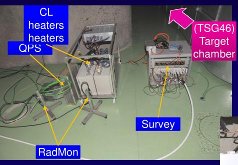
Hottest test area in TSG46:  $\sim 3.3 \text{ Gy}(\text{SiO}_2)/\text{week}$  $\sim 1.8 \ 10^{10}(>20 \text{MeV}) \text{cm}^{-2}/\text{week}$
