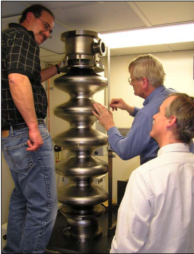
CAVITY PRE-WELD ASSEMBLY
