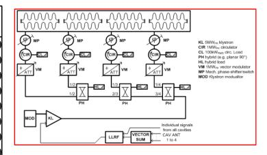
**LPSPL**, but take HPSPL specs for all components incl. klystron, but not klystron modulator
