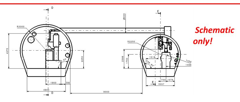
6m klystron tunnel, 4m machine tunnel, separated 9m. All 20m below surface. Surface buildings, above klystron tunnel
