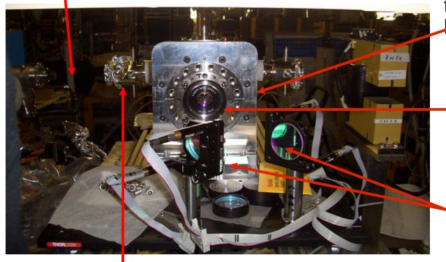
Chamber can be moved along 2 axes transverse to electron beam
