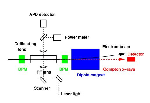
Light steered onto final focus (FF) lens using 2 mirrors
