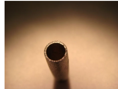
CVD diamond tube fabrication
