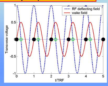
For this reason the RFDs of the CR have been designed with fast filling time, in order to empty the structure as soon as possible. The most simple structure that satisfy this requirement is a TW short structure.
