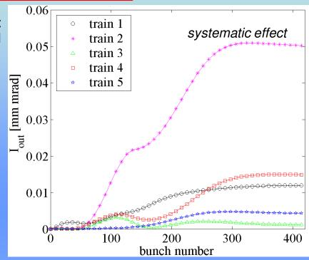
The most synthetic information is given by the **Courant-Snyder invariant of each bunch** after the merging process that can be compared with the nominal projected emittance in case of "systematic" effect, or with the initial invariant in case of injection error.
