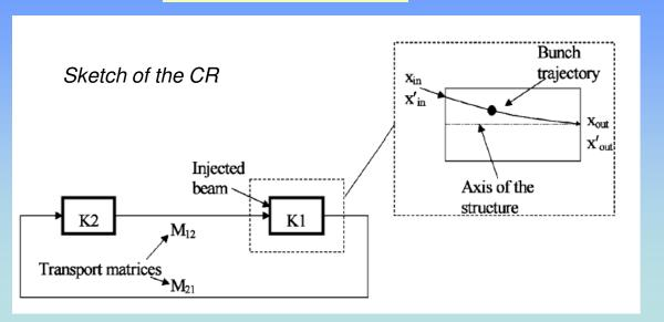
In the CR we can have beam loading effects in the horizontal (deflecting) plane, even in the case of perfect injection since the bunch passes off axes into the deflectors.
