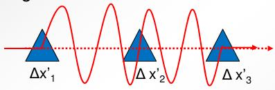
Beam Bump with min. 3 kickers is necessary
