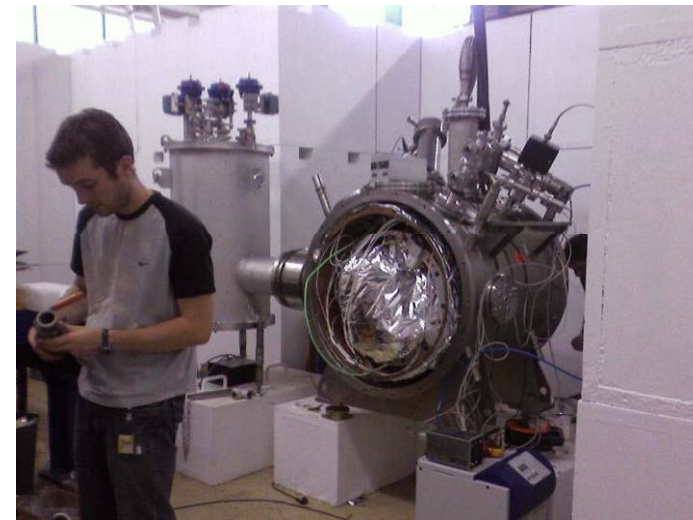
CMO: Horizontal cryomodule for tests
