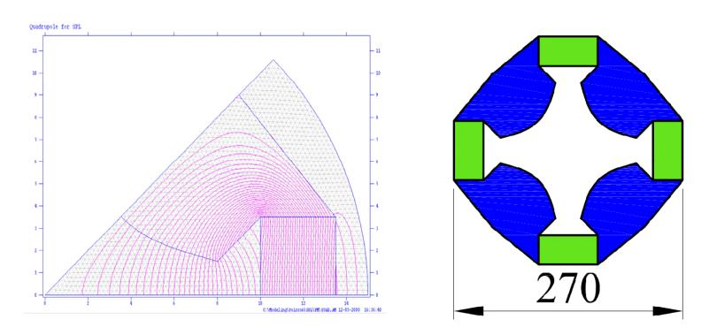
Different configurations are possible with permanent magnets
