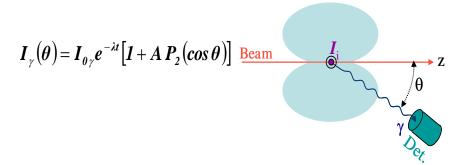
The aligned probe nuclei precess in the "local" field. Emitting  $\gamma$ -rays are detected by one or more detectors placed in the reaction plane.
