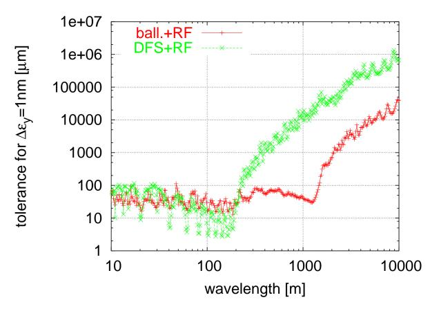
⇒ The alignment tolerance depends on the correction method
