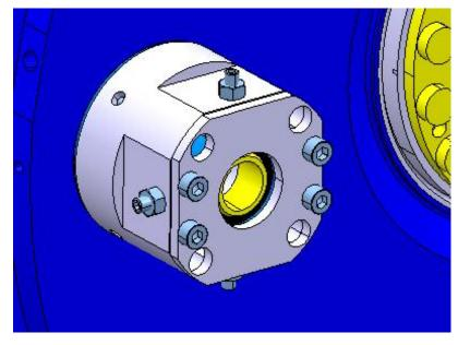
Interfaces foreseen on the helium tank for the second support of the cavity: the « intercavity supporting system »
