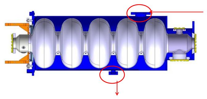
SS CF UHV DN100, tube dia 80 mm -It has been designed to extract the heat in a nominal performance (pulsed).
