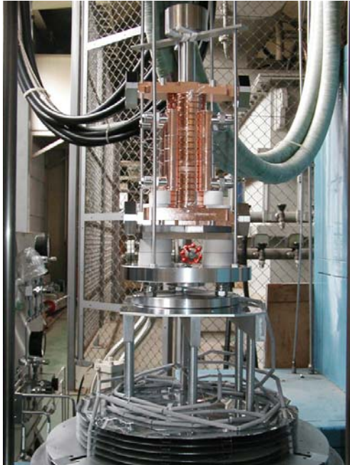
Hydrogen furnace (20cm structure)
