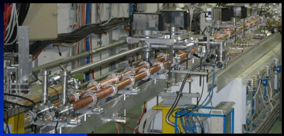
We have TM<sub>01</sub> line (Ø 50 mm) available for up to 160 ns. This was meant for 30 GHz — for 12 GHz we would prefer Ø 90 mm.
