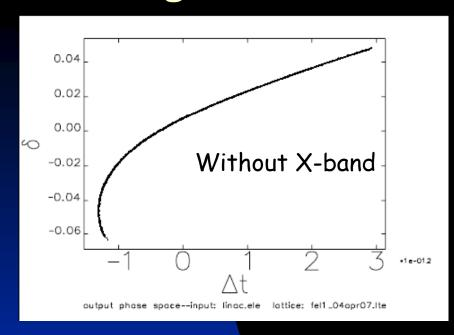
Bunch phase space at exit of 1st bunch compressor.
